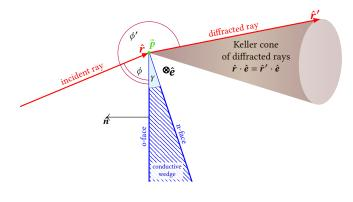
Fig. 4. UTD wedge diffraction.
