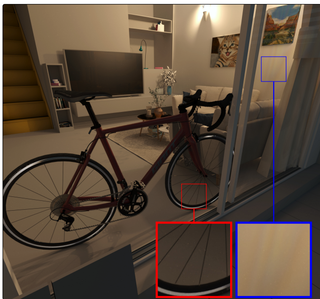
Fig. 10. The bicycle scene from Fig. 1 rendered with indoor lighting that consists of a pair of 3900 K halogen bulbs, as well as late evening sky. Also viewed through a polarization filter. These light give rise to radiation that far less coherent than sunlight, therefore the (red close-up) diffraction grating patterns disappear entirely. (blue close-up) The birefringence effects on the windows also diminish, but remain slightly visible.
